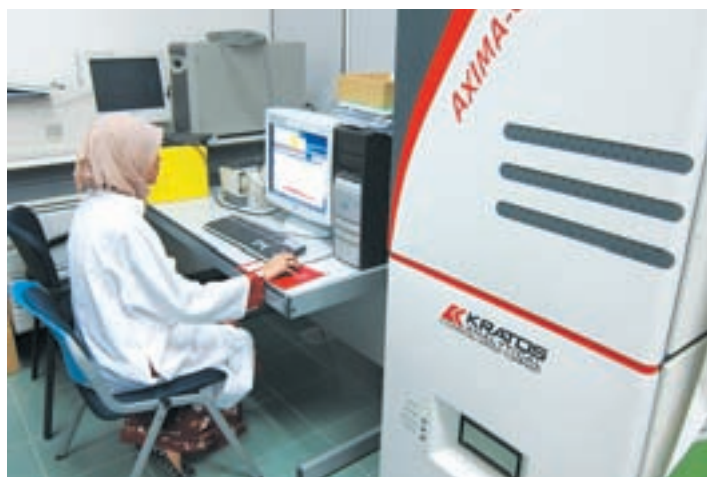
DCC staff using the MALDI-TOF mass spectrometer to analyse the products of collagen digestion using plant-based enzymes
