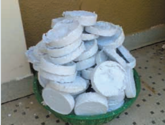
Figure 1: The pulp fibres obtained after the bioenzymatic deinking process
