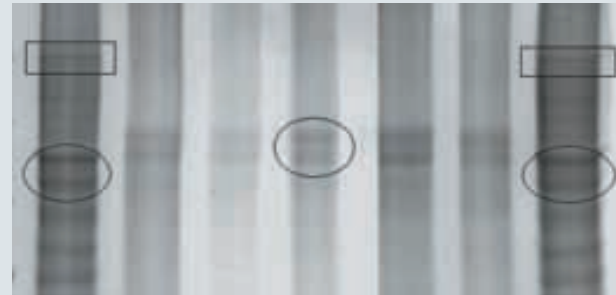
02 Images of bands of bovine and porcine gelatine after gel electrophoresis: (a) and (g) porcine gelatine standard and (d) bovine gelatine standard purchased from Sigma; (b) and (c) bovine gelatine samples (softgel), and (e) and (f) bovine gelatine samples (hard gelatine)
